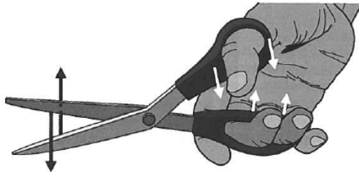
Figure 7-2 Self-help in a scissors. Normal hand action forces the blades' cutting edges together. Left- and right-handed scissors are mirror images of each other, improving the scissors' shearing action for either user.
