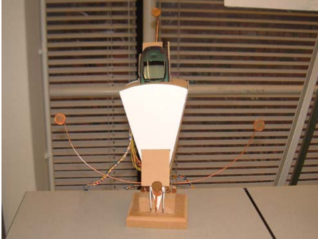
Figure 6: Active telephone cradle with wobble movement.
