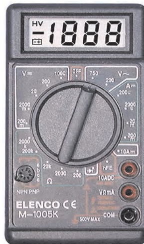
Figure 20.2: A handheld multimeter. On the right the three inputs. The black is the negative or common input, the red one above the positive input for measuring resistance, voltage and low currents. The red input on top is only for measuring high currents. The knob in the middle is used to set the range of the measurement. This can change the values of your input resistance. This multimeter gives its results in 3\frac{1}{2} significant digits. You need to know the accuracy of this multimeter and its input resistance before you can interpret the results.
